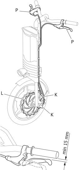
It is extremely important that the distance between the brake lever and the steering lever is not less than 15 mm when the brake lever is retracted as far as possible. Otherwise the braking capacity will not be sufficient
